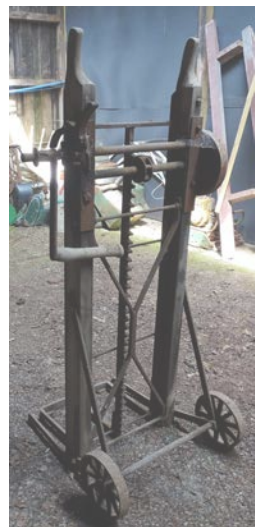
A sack hoist (not a sack barrow) for elevating sacks to the correct height so that the men did not need to bend down
